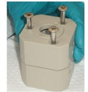
The end of each chamber houses a glass window, which can be removed for easy access to the cornea. An O-ring is also located between the glass window and the chamber to prevent leaks. Two holes on the top of each chamber permit introduction and removal of medium and test compounds and are closed with rubber caps during the treatment and incubation periods.
